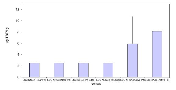
Pit Specific Sediment Chemistry for Tributyltin (TBT) at ESC CMP Vb - May 2025
