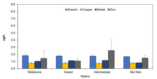
**Figure 7:** Concentration of Arsenic, Copper, Nickel, and Zinc (μg/L; mean + SD) in water samples collected from Routine Water Quality Monitoring for disposal operations at ESC CMP V in May 2025
